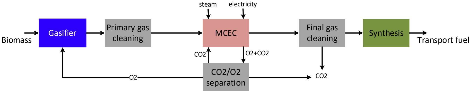
Electrolysis assisted biomass gasification
