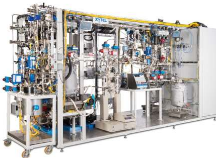
Figure 12. A slurry hydrocracker similar to the one which will be built and commissioned in December 2016 at SP ETC.
