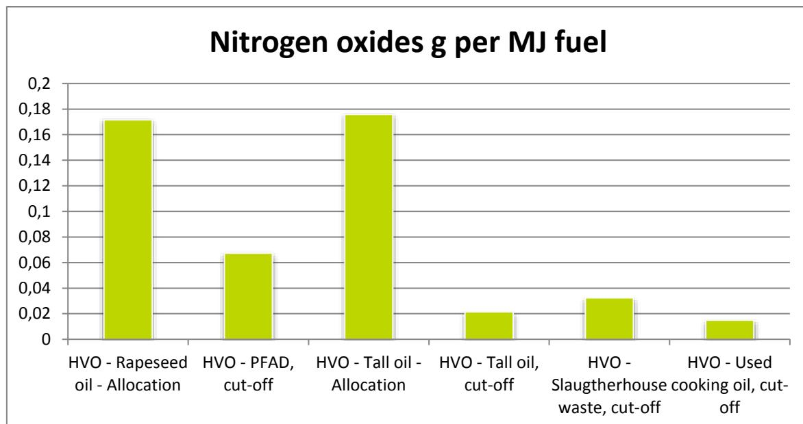
**Figure A1.** Nitrogen oxides Well-to-tank, g per MJ fuel. After the name of each HVO type the approach for the feedstock production is stated. The cut-off approach selected to reflect RED and the economic allocation as a potential alternative. For more details regarding see section 2.3 or the each excel sheets.
