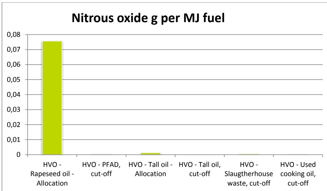
**Figure A3.** Nitrous oxide Well-to-tank, g per MJ fuel. After the name of each HVO type the approach for the feedstock production is stated. The cut-off approach selected to reflect RED and the economic allocation as a potential alternative. For more details regarding see section 2.3 or the each excel sheets.
