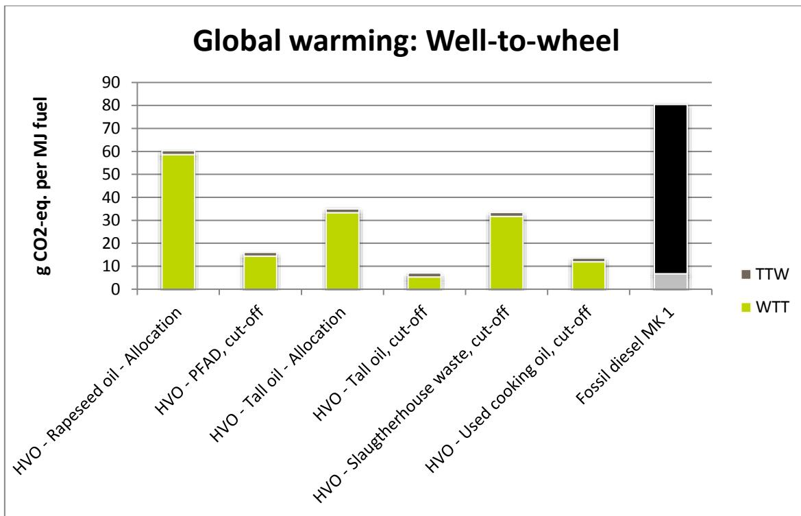
**Figure 2. Global Warming Potential: Well-to-wheel with fossil diesel MK1 as a reference.** After the name of each HVO type the approach for the feedstock production is stated. The cut-off approach selected to reflect RED and the economic allocation as a potential alternative. For more details regarding see section 2.3 or the each excel sheets.
