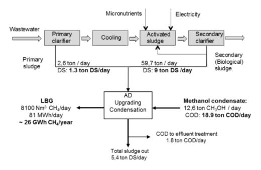
Figure 4. Schematic overview of the external wastewater treatment with the addition of an upgrading procedure to produce LBG from the DS in the primary- and secondary sludge and from the COD in the methanol condensate.
