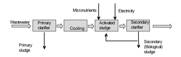
Figure 2. External wastewater treatment in pulp and paper mills.
