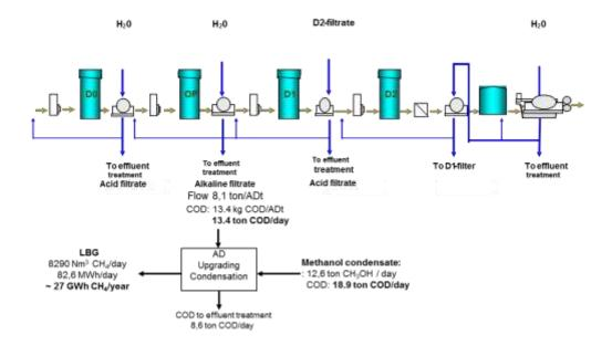
Figure 3. Schematic overview of a bleach plant for a typical kraft pulp mill in Scandinavia with the addition of an upgrading process of the present COD in the alkaline filtrate and in the methanol condensate to produce LBG.
