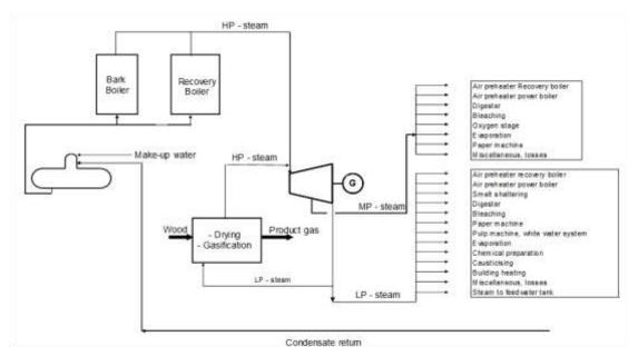
Figure 10. Suggested integration possibility of a drying- and gasification step into a typical steam balance of an average integrated pulp- and paper mill.
