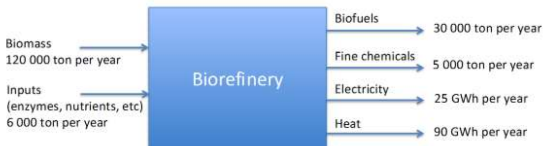
Figure 6.1. Example of a generic biorefinery. The biorefinery is assumed to be energy self-sufficient, i.e. the required process energy is produced internally from biomass and/or via energy recovery within the plant. All numbers are for illustrative purposes only and are not intended to reflect a real situation.
