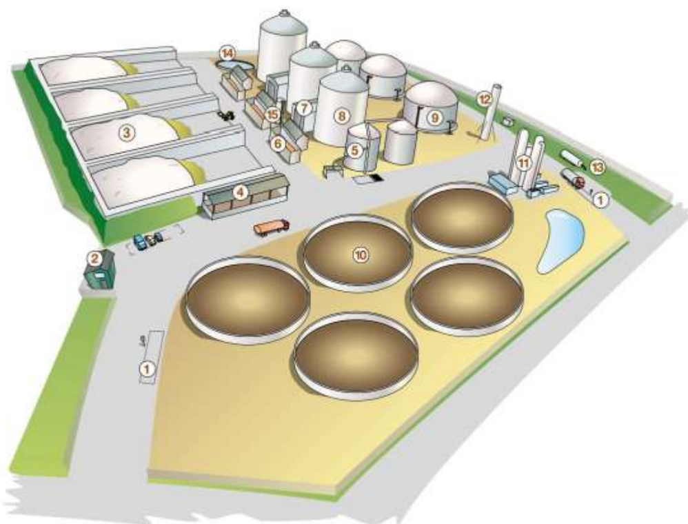
Figure 1 Overall layout of Jordberga biogas plant where 1. Weighing station, 2. Office and control room, 3. Bunker silos, 4. Roof covered area for dry substrates, 5. Tower silos, 6. Feeding containers, 7. Machine buildings, 8. Main digesters, 9. Post digesters, 10. Digestate storage, 11. Biogas upgrading, 12. Flare, 13. Propane tank for addition before injection to gas grid, 14. Storage for rain-leachate water, 15. Tank for liquid substrates.
