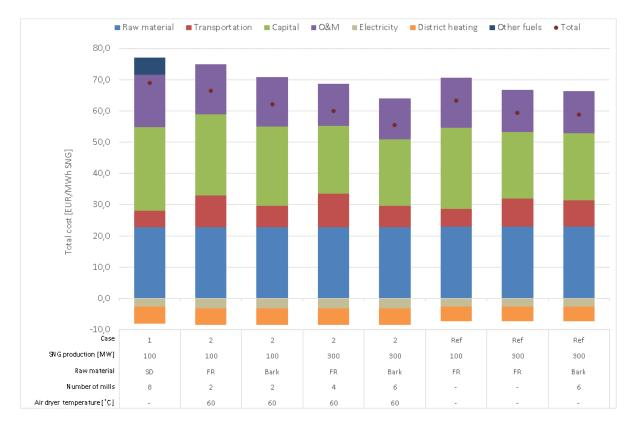
Figure 19. Total SNG cost showing the contribution from the cost of raw material, transportation, capital, O&M and other fuels as well as the net revenues for electricity and district heating.
